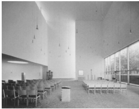
2 Büttner Neumann Braun, St Canisius Church, Berlin, 2003 A clear glass wall allows the church interior to open out onto an enclosed space outdoors. Additional direct daylight comes from a band of light and indirect light from a translucent glass membrane behind the altar. The mean daylight factor lies between 2.1 and 3.2 per cent.
